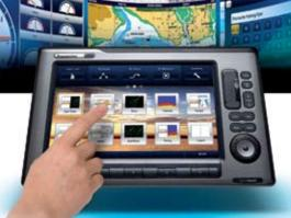
Scrolling, panning, function selection and every-day navigation essentials are literally at your finger tips. Use the slick touch screen for guickness and ease in calm conditions or revert to hard keys when the rain starts pouring and the going gets rough.
