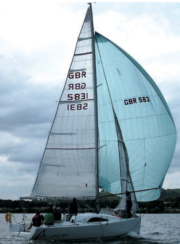
ABOVE The rig is a simple non-overlapping twin spreader alloy 9/10ths rig, nicely made by Soromap.
