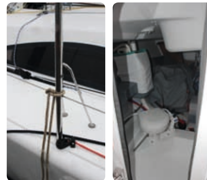
ABOVE LEFT The stanchions have two optional heights for guardrails for optimal hiking.
